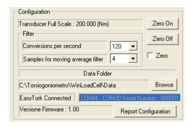
The window **Filter** allows you to define the operative mode of the EasyTORK transmitter.
