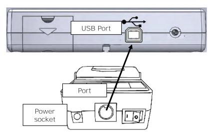
**NOTE:** Thermal printer needs to be powered by adapter
