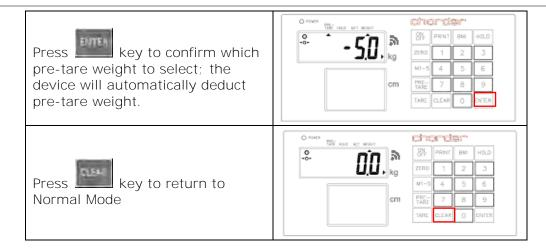
NOTE: Pre-tare weight must be under max capacity, otherwise screen will show 0.00 after key is pressed, and the operator will have to re-input pre-tare settings.
