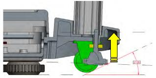
Ensure stability foot is retracted before using castor wheels
