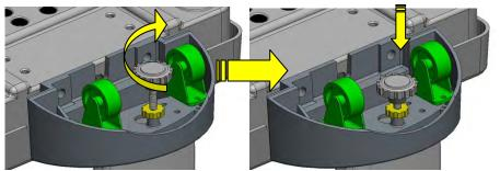
Note: rotate counter-clockwise to extend, clockwise to retract
