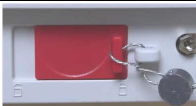
Locked with Wire Seal
