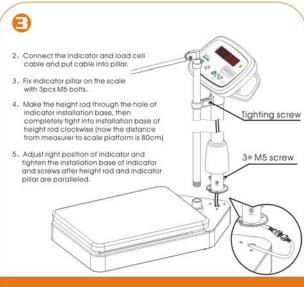
Notice: 1. Put the scale on flat floor during installation
